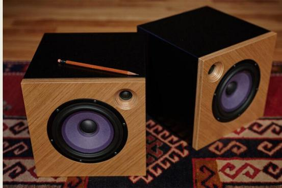
The Orangutan micr/O was designed alongside the O/baby and uses the same internal components. This perfect little sealed cube will fit anywhere, with response tailored to sound just right in a bookcase, record shelves, a desktop, or on a side table. With a horn-loaded .75" textile dome tweeter and 7" paper woofer.
